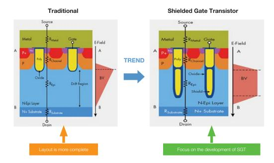
SGT MOSFET Significantly reduce losses and improve efficiency
