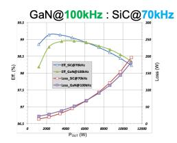
12 kW: V<sub>IN</sub>:240 V, V<sub>out</sub>: 400 V Half-bridge Synchronous Converter
